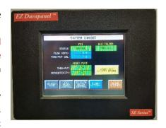
operation on either batch (flow sensors standard), resistivity or both. The AB 10/100 IP Ethernet Network Connection port is standard for building management capabilities. Custom Programming and alternate communication protocols are available.
